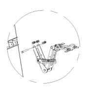
1.Fix and ensure the top mounting stable to the top bracket by M8\*20 bolts and nuts.
