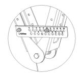
6.Adjust the downtilt angle to X degree, then lock the bolt.
