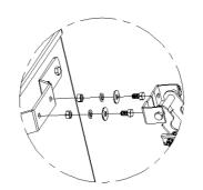
1.Fix and ensure the top mounting stable to the top bracket by M8\*20 bolts and nuts.
