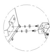
2.Fix and ensure the bottom mounting stable to the bottom bracket by M8\*20 bolts and nuts.
