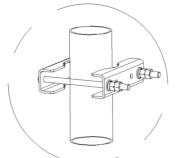
5.Fix upper clamp at the mounting pole, then fasten all the nuts tightly.
