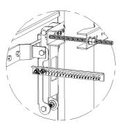
3.Fix the lower clamp at the proper position 4.Adjust the downtilt angle to 0 degree. of the mounting pole.
